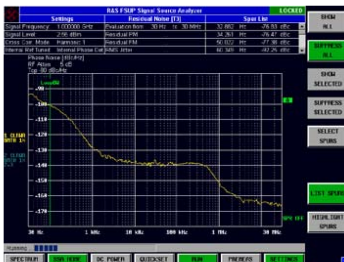
Interference can be suppressed to obtain a spurious free measurement trace for documentation.
