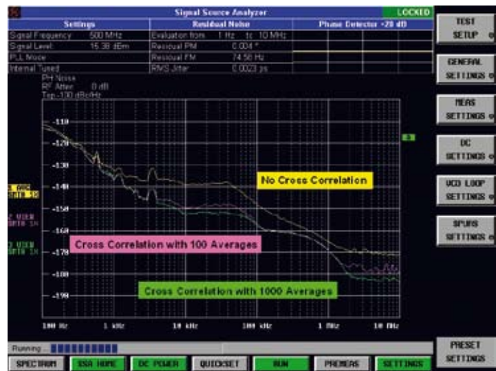
Improvement of phase noise sensitivity achieved by means of cross-correlation. A phase noise measurement is shown without cross-correlation (yellow trace) and with cross-correlation (100 and 1000 averages).
